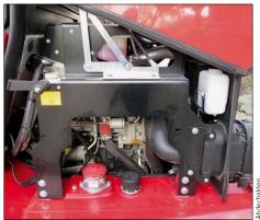
A hood which can be opened wide makes maintenance work easily
