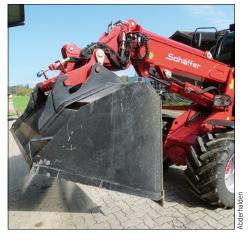
The rapid coupler holder is extremely robust and the hydraulic interlock is top notch. Practical detail: Schäffer devices have two upper coupling points. This enables a larger tipping angle whenever it is required. Another detail: The Schäffer holder is compatible with the Kramer Allrad holder.
