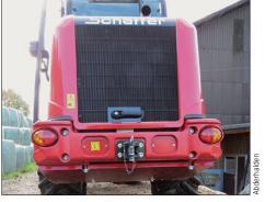
As additional weight a 200 kg plate is fitted under the rear end. The light unit is fitted in such a way that it is very well-protected.
