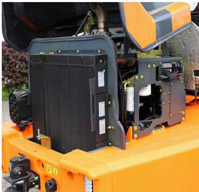
The 75hp Deutz engine of the latest generation complies with the strict Emission Stage V standards. Alle service points are easily accessible.
