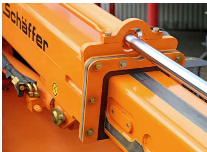
Additional protection against thawing salt is provided by the sealing of the telescopic arm.
