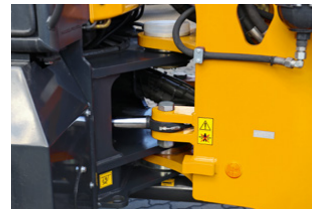
The beefy articulation is heavy-duty and maintenance-free. Tight steering angles make for high agility.
