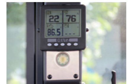
New information display in the B-column for the exhaust gas system for 8600 and 9600 series loaders
