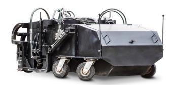
With the paddock cleaner, mucking out is done quickly. It is ideally suited for mucking out all hard surfaces such as horse paddocks, hard pastures, trails or yard areas. The six reinforced rubber lips collect the manure and transport it into the collection container. The hopper can then be emptied on the manure plate. This technique saves valuable time and leaves a clean result.
