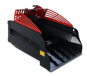
The mini straw spreader is the perfect addition to the Schäffer 1622 for distributing straw in stables. The straw is conveyed to the hydraulic opening roller via a mechanical feed roller. From there, it reaches the blower that can spread straw up to 10 metres away.
