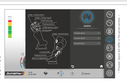
In the joystick menu, three function buttons can be assigned individually depending on the machine equipment. At the same time, the button assignment can be read. The load display at the top left always remains visible, as does the status bar in the lower section.
