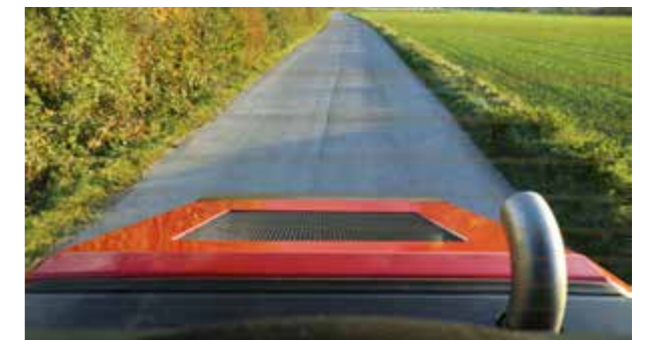
The rear sloping bonnet ensures a better view of the working area behind the machine.
