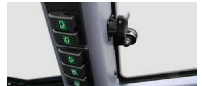
Switch bar, electric plug
