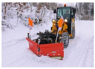
The Vario snow plough features two hydraulically swivelling wings. Snow can be cleared in the V, Y or diagonal position. This snow plough is therefore the ideal companion for clearing snow from footpaths, cycle paths and roads.
