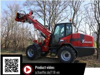
The hydraulic pruning saw is used to efficiently cut back dense hedges or trees. Three large saw blades, each with a diameter of 60 cm, cut branches up to 15 cm thick. The sturdy mounting frame allows for hydraulic lateral displacement and stepless lateral swivelling.
