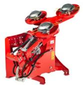
The fence trimmer cuts around fence or crash barrier posts, freeing them effectively and quickly from overgrown grass and weeds. Operated by the loader, the disc unit reaches under the fence and rotates on its axis the moment it contacts the post, cutting and freeing it from all grasses and weeds. The plastic rails protect the post from impact damage.
