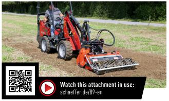
The hydraulic soil reversal tiller is the reliable partner for seedbed preparation in garden landscaping. The milling blades, which rotate against the direction of travel, pick up the soil and throw it against a sieve grid. Coarse components are sieved out and buried. The soil, freed from grasses and plant residues, lies on top as a top layer. Thanks to the crumbler roller, the soil is reconsolidated.
