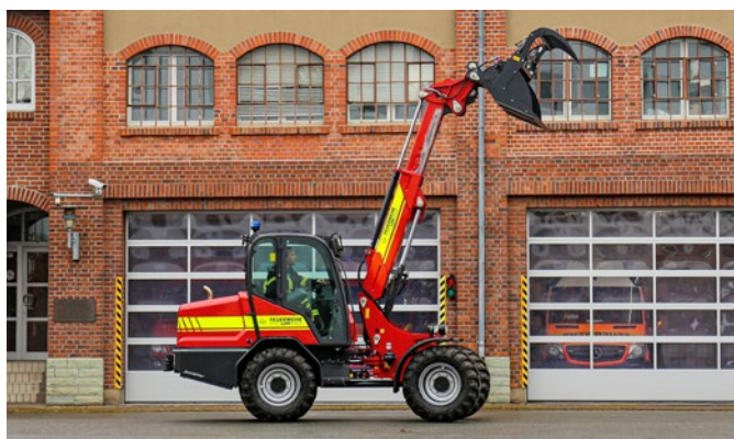
The Schaeffer telescopic wheel loader 6680 T has an operating weight of roughly 6 tonnes and a lifting height of 4.95 metres.
