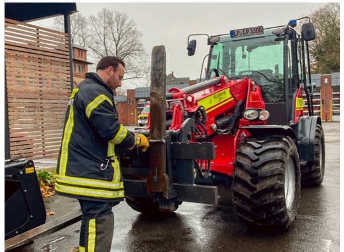
The tines of the pallet fork can be folded up to enable safe road transport to the incident site.
