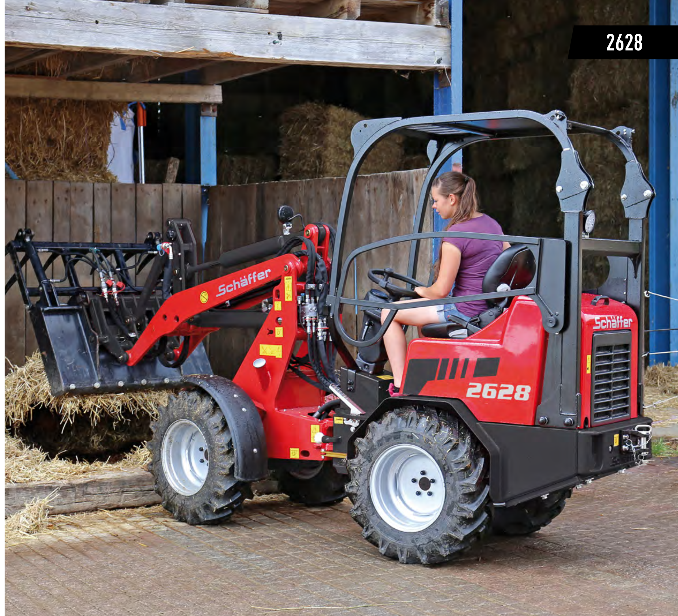
The motor room opens forwards. This makes all service points easily accessible from both sides of the machine.
