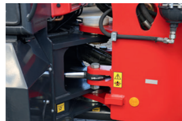
The articulation joint is very strong and maintenance free. Two steering cylinders give perfect control.
