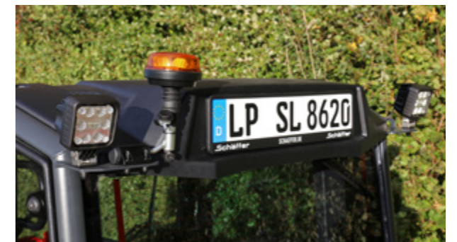
To the rear, there is also space for up to four working headlights; alternatively, one headlight can be replaced by a beacon light.
